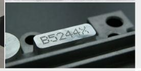
The XF510m Dot peen marking solution range marks all materials and part shapes up to 62 HRC: raw, machined, painted, flat, convex, concave etc.
