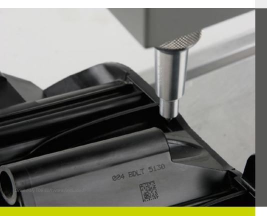
Integrable electromagnetic micropercussion marking solutions
